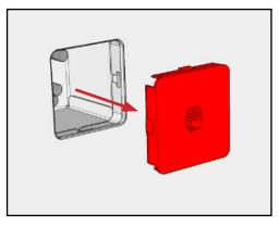
12. Carefully remove the finishing guard from the fixture opening.
