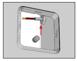
4. Bring low voltage wiring from the remote power supply to the housing and feed low voltage wires through the cable gland opening.
