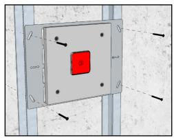
2. Fasten the bracket to the framing using the screws provided with the bracket.
