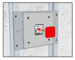
**7.** Safely remove the fixture and insert the finishing guard into the fixture opening to prepare for finishing.
