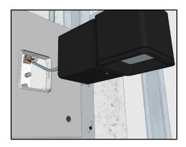
5. Make the **low voltage electrical** connection. No conduit knockout is needed as this is a low voltage product.
