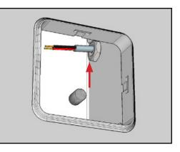
**4.** Bring **low voltage** wiring from the remote power supply to the housing and feed **low voltage** wires through the cable gland opening.
