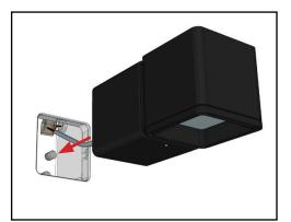
13.Make the low voltage electrical connection.
